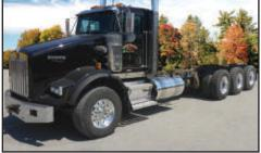
2014 T800 Kenworth, 16K front 69K rears, ISX Cummins 550 HP Jake Brake Cruise.
