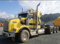
2015 T800 Kenworth, 20K front 69K rears, ISX Cummins 550HP Jake Brake Cruise.
