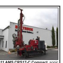
2011 AMS CRS17-C Compact, sonic drillhead, John Deere 4045 diesel, 173 hp, hyd. hoist, rod clamp, wireless remote, water pump, vibration: 20,000 lbs - 28,000 lbs, feed system: 12' and 8' stroke, pullback force: 13,000 lbs, carrier has 4.6 psi ground pressure, 1545 hours......\$199,500 909-600-7555
