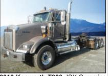
2013 Kenworth T800, ISX Cummins 550 hp, 16K front 46K rears, 4-way lockers, full-double frame, Jake Brake, Cruise, 382,417 total miles.
