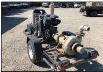
Trailer mtd. mud pump, 2007 Tier 1, 100 hp 4 cylinder Perkins turbo diesel (estimated 3000 hrs), Rockford PTO in out clutch, 4x3 Mission Magnum sandmaster with mechanical seal, 25 gallon fuel tank, custom built trailer.....\$27,500 707-255-7923
